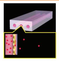
Blood capillary networks consisting of bilayered structures of human endothelial cells and smooth muscle cells are prepared inside biodegradable hydrogels by a combination of uniaxial tubular microchannel fabrication and hierarchical cell manipulation. These blood capillary analogs, possessing blood barrier functions similar to native blood capillaries, can be useful for in vitro permeability assays of drugs and as drug delivery carriers.
