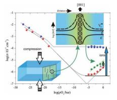
One-dimensional defects created in TiO<sub>2</sub> single crystals by uniaxial pressure strongly increase the conductivity parallel to the formed dislocations (at oxygen partial pressures from 10<sup>-5</sup> bar to 1 bar) and even change the type from predominantly electronic to ionic. This can be explained by the accumulation of positive point defects in space charge zones adjacent to negatively charged dislocation cores.
