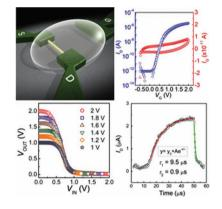
Flexible ZnO nanowire-based field-effect transistors (FETs) are built with a composite solid polymer electrolyte as the gate insulator to ensure battery-compatible, low voltage operation ( $\leq 2$  V). Long-term, stable performance of the nanowire FETs in air is demonstrated. Even though electrochemically gated, the in-plane device geometry already shows an extremely fast switching of >100 kHz, which should increase further for the topgate configuration.
