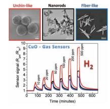
High-performance gas sensors based on CuO hierarchical morphologies with in situ gas sensor comparison are reported. Urchin-like morphologies with high hydrogen sensitivity and selectivity that show chemical and thermal stability and low temperature operation are analyzed. The role of morphological influences in p-type gas sensor materials is discussed.
